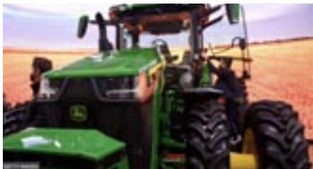
Cameras—visible here in the lower front of the vehicle—detect objects as the tractor tills
